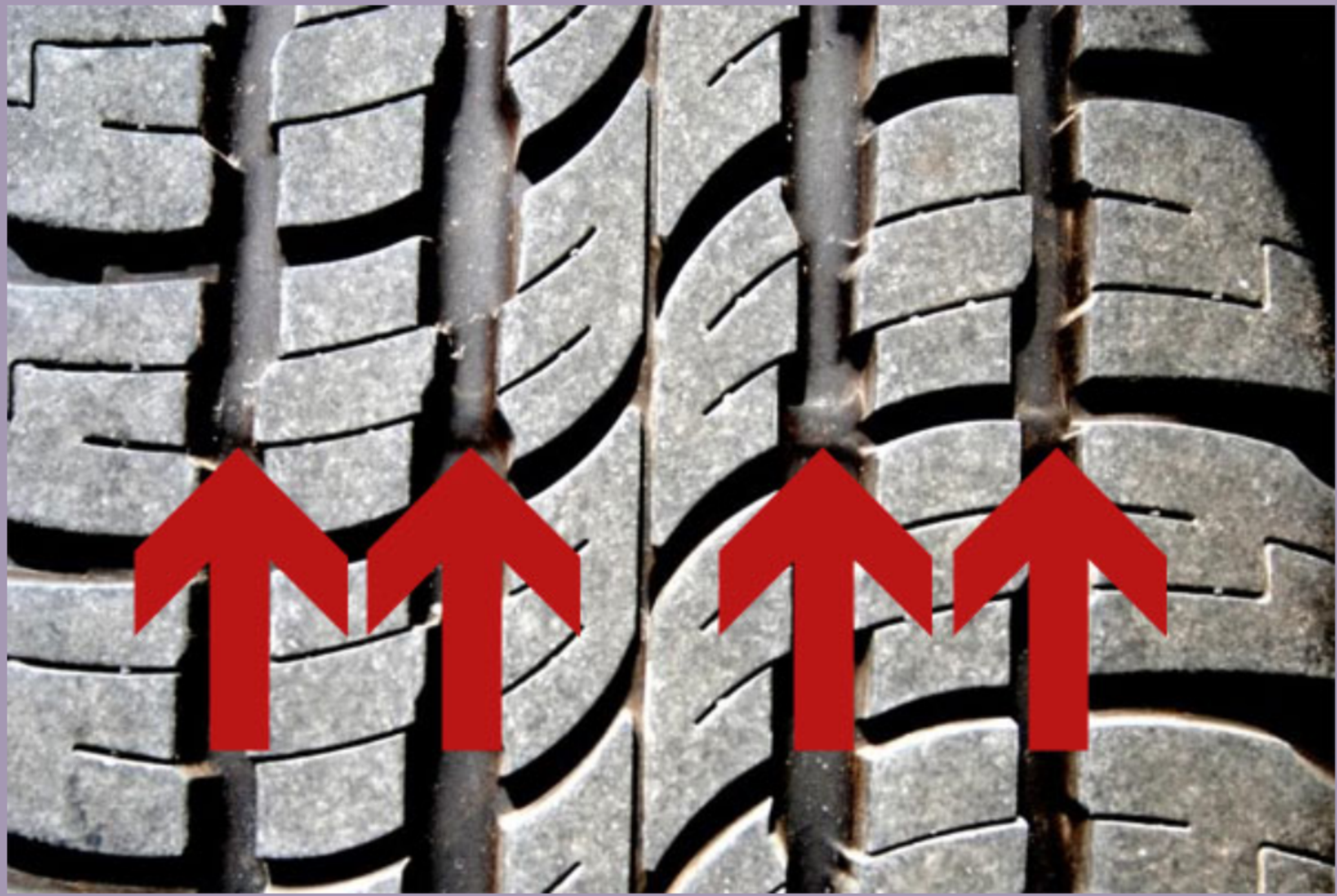
Enlarged image of a tire tread shows characteristics unique to the mold used to create this tire (red arrows). (Courtesy of John Black, Ron Smith & Associates)
