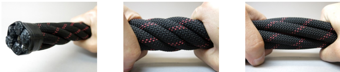
Figure 1: Hand model showing nominal lay length (left), closing twist “ +\omega ” (middle) and de-twisting “ -\omega ” (right)
